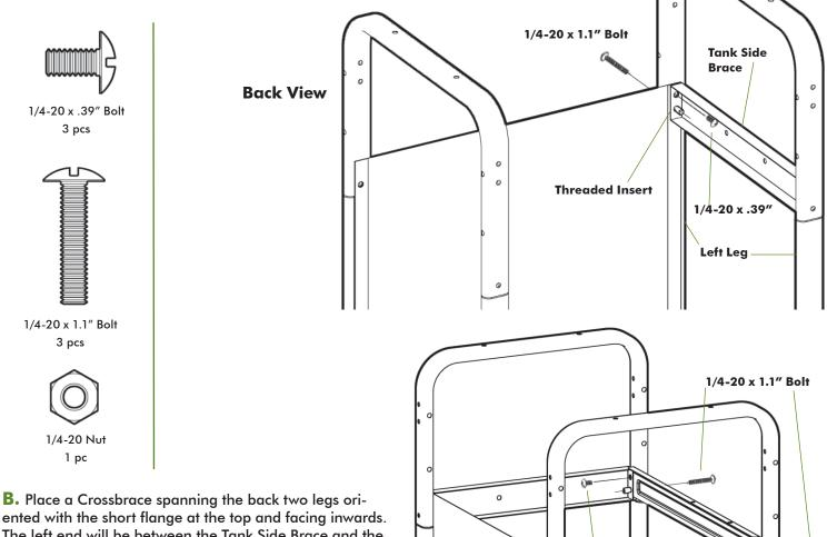
ented with the short flange at the top and facing inwards. The left end will be between the Tank Side Brace and the rear leg of the U-Frame so that the holes in all parts align.
